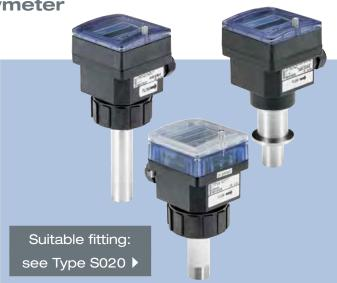
The electromagnetic flowmeter 8045 is made up of an electronic module including a backlit display, operating keys for configurations and a sensor consisting of PVDF or stainless steel material. It has been designed to measure a flow rate of neutral and slightly aggressive fluids with a conductivity of more than 20  $\mu\text{S/cm}$  in DN06... DN400 pipes.
