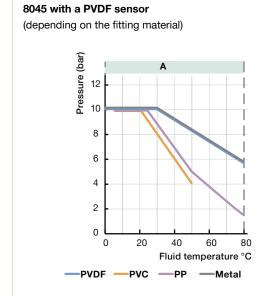
A : Application range for complete device (fitting + flowmeter)
