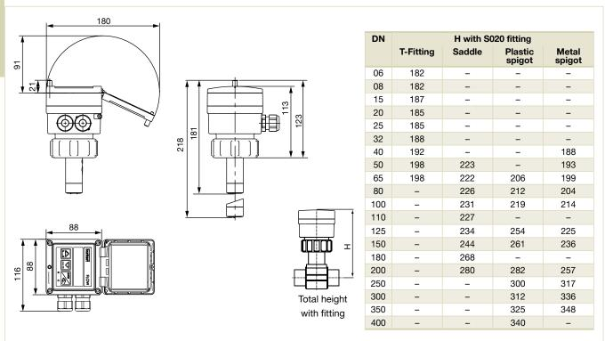
**Note:** The Type 8041 can easily be installed into any Bürkert Insertion fitting system (S020) by just fixing the main nut. The length of the sensor armature depends on the nominal size of the fitting used.
